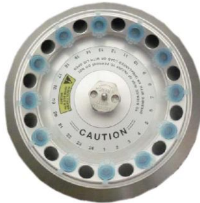
Figure 1. Loading the rotor to achieve balance
