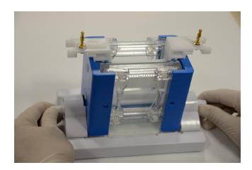
7. With the cam handles facing directly downwards, rotate the cams in the opposite direction 180° or until the insert has tightened down onto the gasket. **Do not overturn as this will cause the glass plates to push upwards and the assembly will be more likely to leak.**
