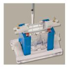
6) Once set, transfer to tank and fill inner and outer chambers with buffer.
