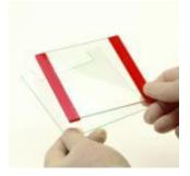
2. Assemble the glass plates so that the bottom of the glass plates and the spacers are perfectly aligned. For triple plate sandwiches, the free spacers need to be perfectly aligned which is best performed using a small spacer or comb to push the spacers apart. Notched glass plates with bonded spacers do not need
