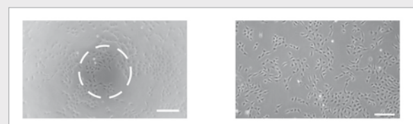
Beam path with meniscus No alignment, bad phase contrast.
