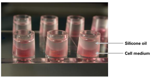
μ-Slide VI <sup>0.4</sup> with silicone oil (ibidi Anti-Evaporation Oil) inside the reservoirs, which is used to decrease evaporation in non-humid environments, e.g., on the microscope.
