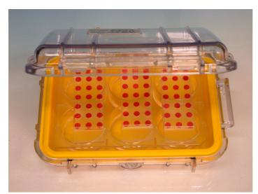
An Olaf Chamber with a µ-Slide 18 well inside. A water-filled 6 well plate provides humidity.
