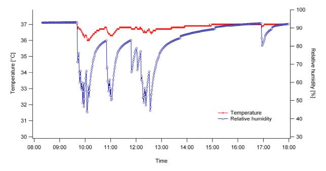
The above graph shows the temperature and humidity inside a  $\rm CO_2$  incubator over a 10 hour day, during and after briefly opening the door. The graph shows only minor differences in temperature over the day, i.e., between 36°C and 37°C. However, it shows significant differences in relative humidity over the day, i.e., between less than 50 % and the steady state of 93 %. An important fact to note is that this incubator had not been opened all afternoon, except briefly just before 5 o'clock.
