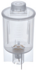
DIS-300-S-M.10 Dissolver tube Volume: up to 300 ml Application: Crushing and dissolution of tablets and dragées. This tube is equipped with a dissolver blade and opens up new application fields. It was especially designed for dissolving samples in different solvents. Ident. No. 0020016318
