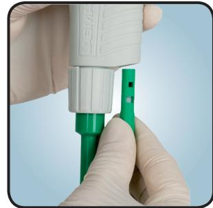
The adjustable ejector height system – to accommodate virtually all brands of tips
