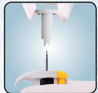
Insert the calibration key and locate in the key slots. The calibration key is delivered with the pipette.
