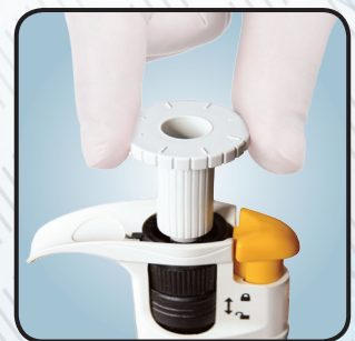
Turn the key to increase or decrease the display volume. Refer to the user manual for details.
